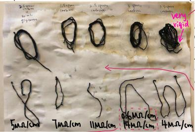
Observations: Resistance values along the yam one far from consistent because the liquid was not perfectly mixed before extrustion.
