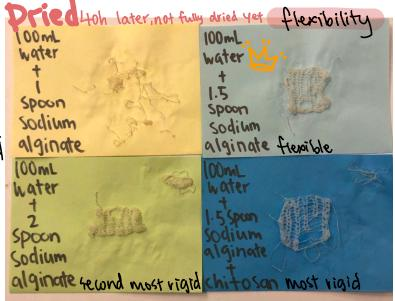
Recipe: 100 mL water Sodium talginate conductive powder 4.24.2 bioplastic yarns of different compositions Colored
