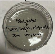
I spoon instead of the usual 1.5 spoon to try if conductivity could be improved. This was a mistake because although your diameter increased, it broke two easily during the knitting process.
